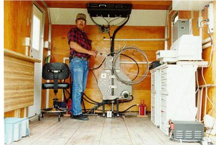
For production testing the miniature CPT system may be mounted on the front of a four wheel drive vehicle. This allows additional freedom of vehicle type and provides easy access to sites near structures or in confined spaces.
