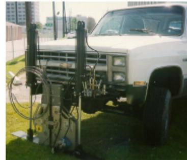
This single piece coiled thrust rod minimizes the complexities of waterproofing of the cone electronics by eliminating threaded connections found on conventional cone penetrometer systems. The probe tip is equipped with an electronic load cell that measures resistance offered by the soil during intrusion. The shaft of the probe is equipped with a friction sleeve to measure the local friction with surrounding soil.
